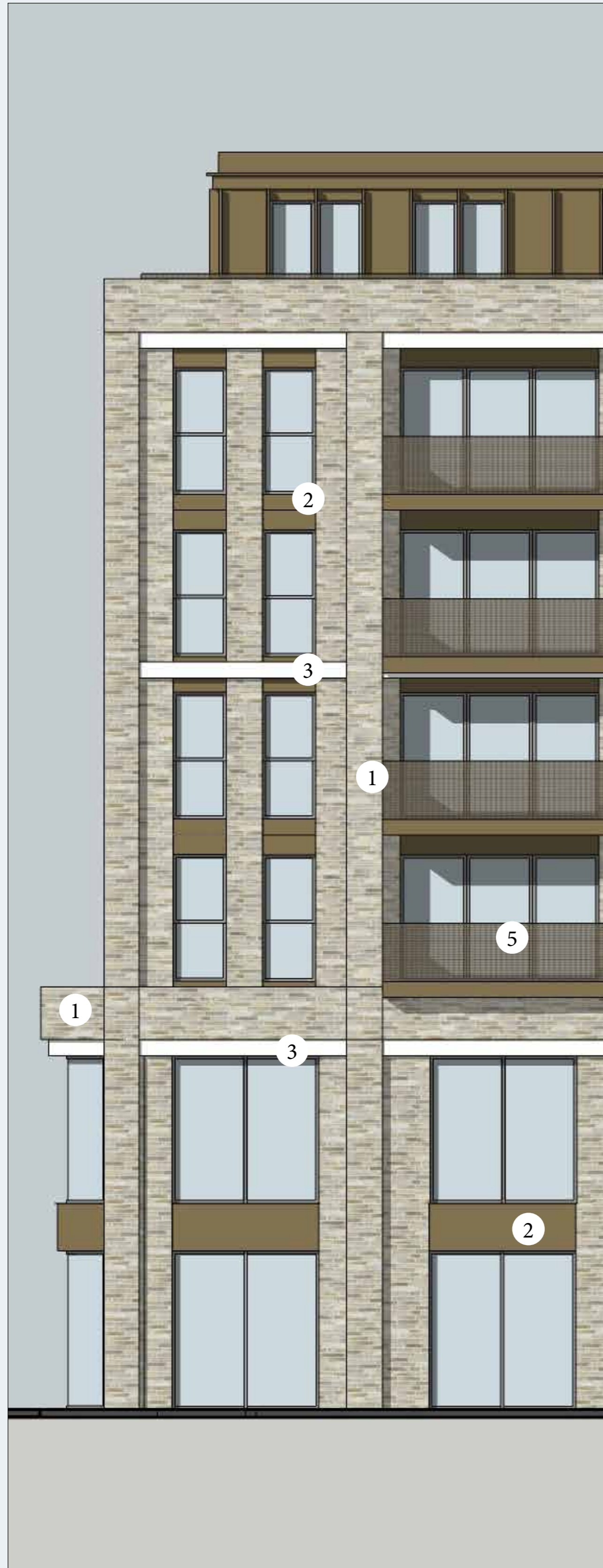
Block A - Section of east facade
